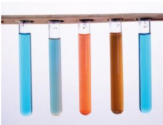
Figure 2.12 The test for reducing sugar. Far left tube is a control with distilled water; the subsequent tubes (left to right) contain 0.1%, 1%, and 10% glucose solution. Far right tube contains sucrose – not a reducing sugar so no colour change seen
